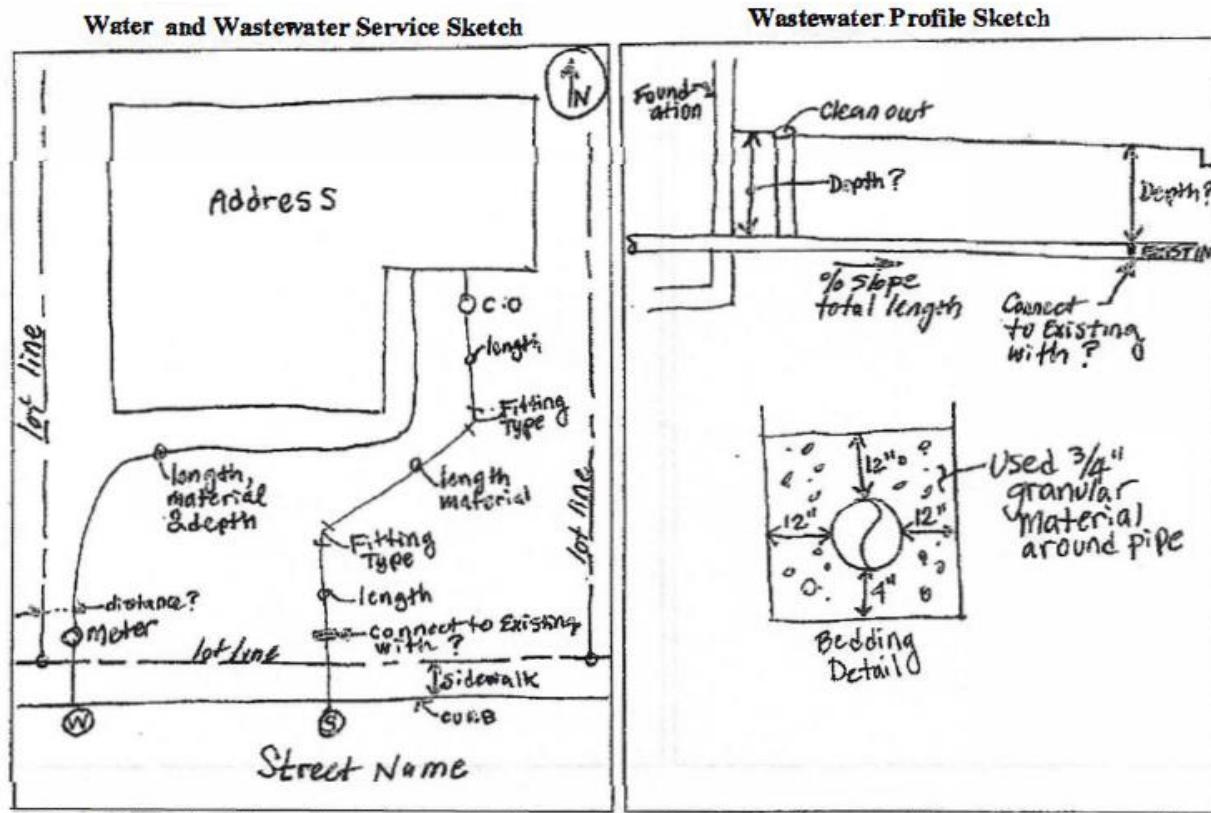
**Sketch Criteria:** Show North Arrow, lot lines, piping lengths, piping material types, depths, couplings, fittings, clean-outs, curb stop box or meter pit referenced from two locations, sidewalk with "W" and "S" each location, foundation, ground level, piping slope.
