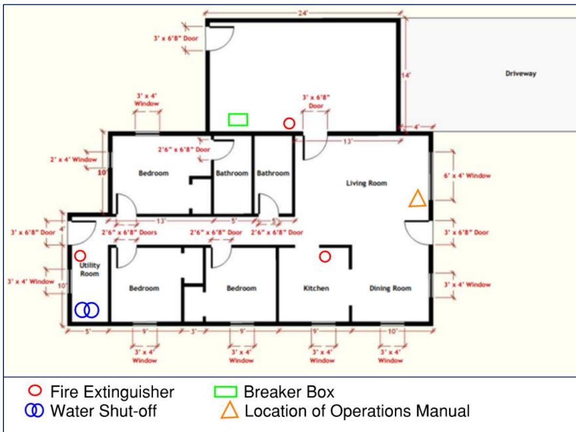
\*Symbols used to show fire extinguishers, breaker box, and water shut-off are for example only and can be modified.
